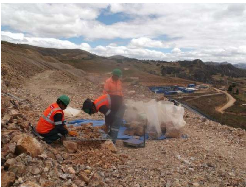
Figure 1: In situ determination of the global particle size distribution of coarse granular materials
