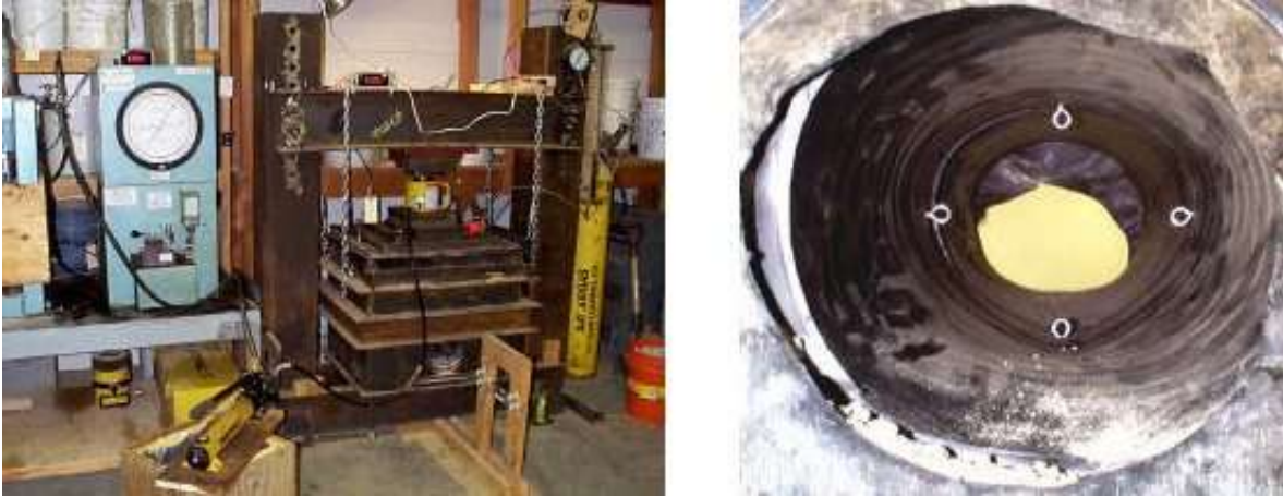
Figure 6: (Left) Pipe deflection test apparatus. (Right) Pipe after 2,000 kPa loading
