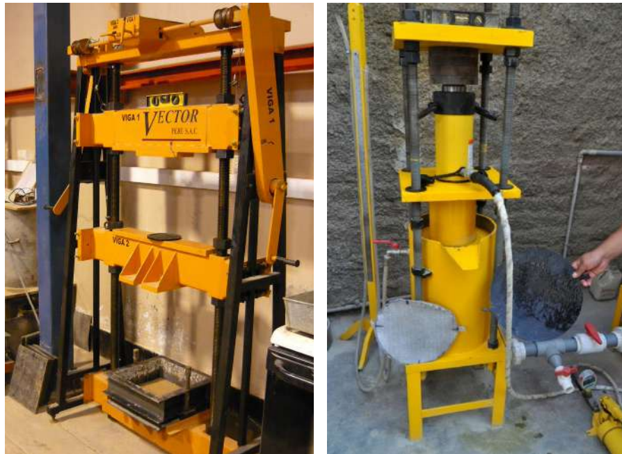
Figure 2: Equipment for puncture testing. (Left) Square box and (Right) Cylindrical box
