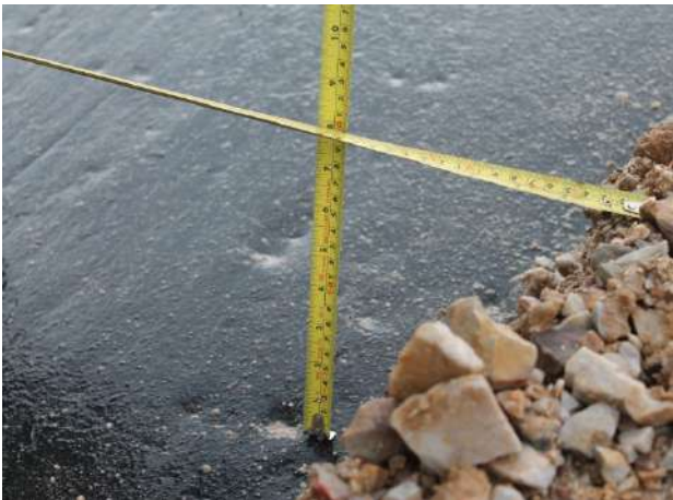
Figure 9: Overliner thickness verification
