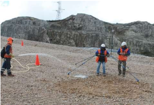
Figure 7: Anomaly verification (leak location)
