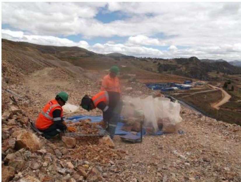
Figure 1: In situ determination of the global particle size distribution of coarse granular materials
