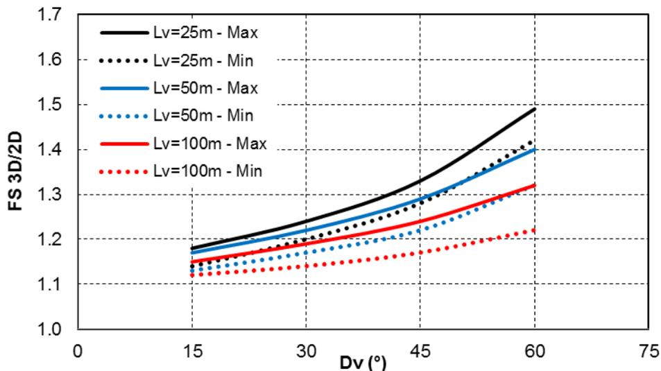
**Figure 5: 3D/2D FS trends for different  $L_v$  and for  $L_c=100m$ ,  $H=150m$  and interface I1**
