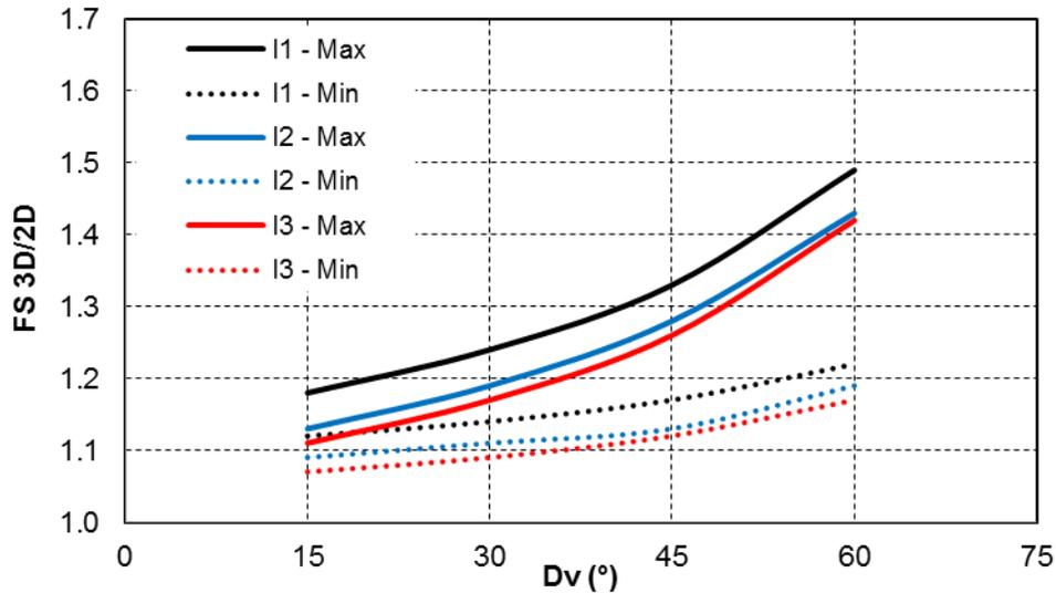
**Figure 7: 3D/2D FS trends for different interface shear strength envelopes and for H=150m**
