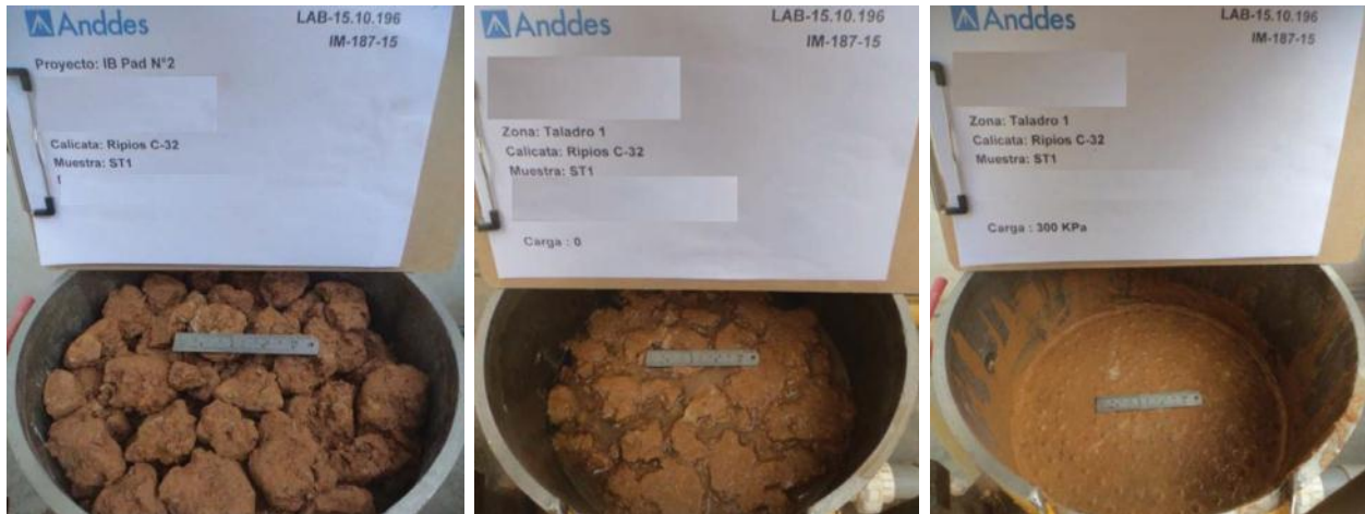
Figure 5: condition of sample ST-SD a) before first test b) after first test 0 kPa c) after second test 300 kPa
